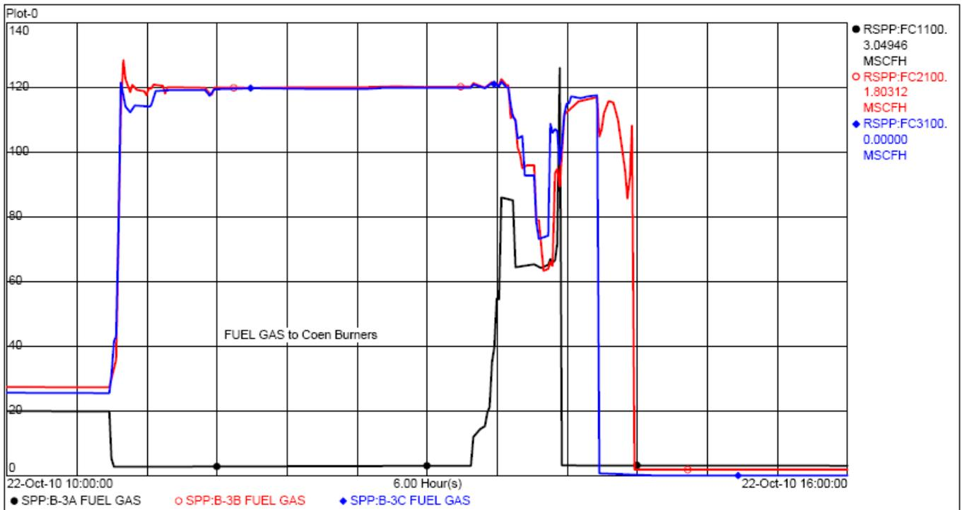
Steam Power Plant Fuel Gas Flow to COEN Duct Burners A, B, and C
