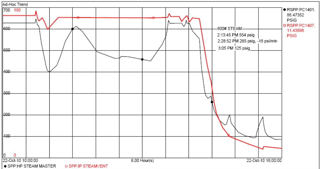
Steam System Pressure: 600# (High Pressure, HP) and 150# (Intermediate Pressure, IP)
