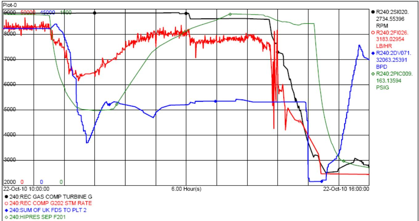
Unit 240 Recycle Gas Compressor RPM & Steam Rate versus Feed Rate & Pressure
