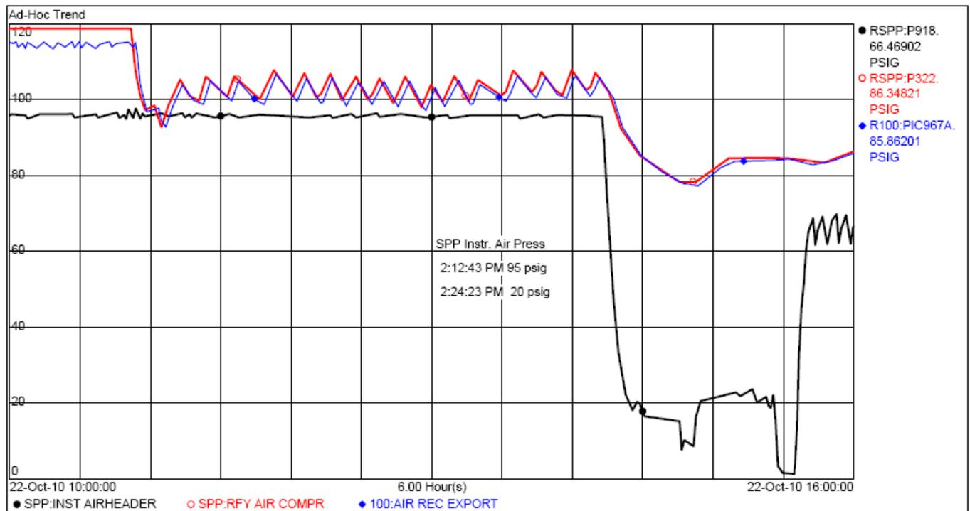
Refinery Air Pressure versus Steam Power Plant Instrument Air Pressure
